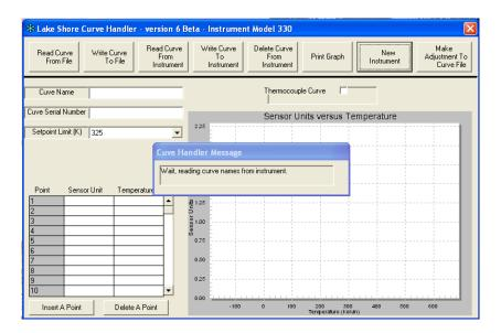
11. To verify that the curve was written correctly or to read a curve that is stored in the instrument select the **Read Curve From Instrument** button. Choose the curve to be read from the drop down box then click **OK**.
