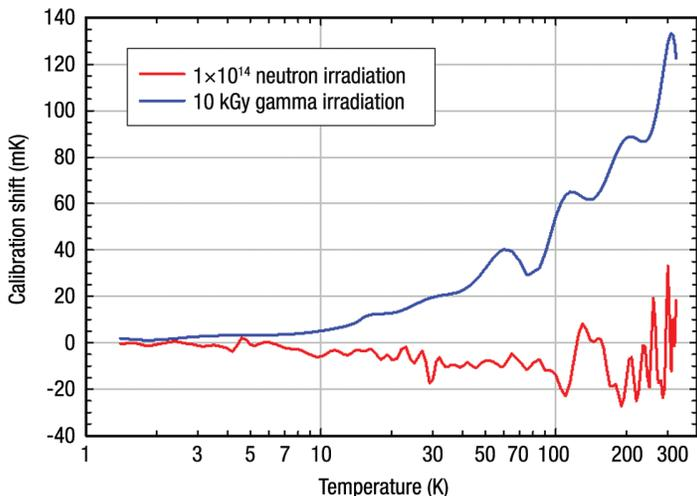
**FIGURE 11.** Calibration shift induced on Model CX-1050 Cernox sensors by room temperature irradiation at  $1 \times 10^{14}$  n/cm<sup>2</sup> (red line) and 10 kGy gamma radiation (blue line).
